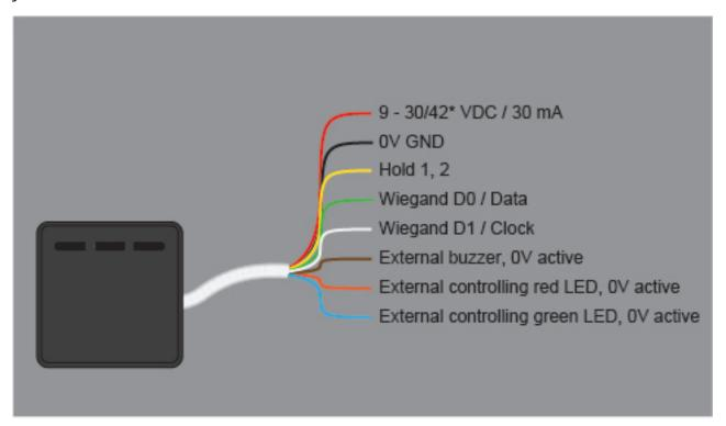
**\*Note:** The P1200 reader can withstand 9-30 VDC, while the M1200 can withstand 42 VDC.
